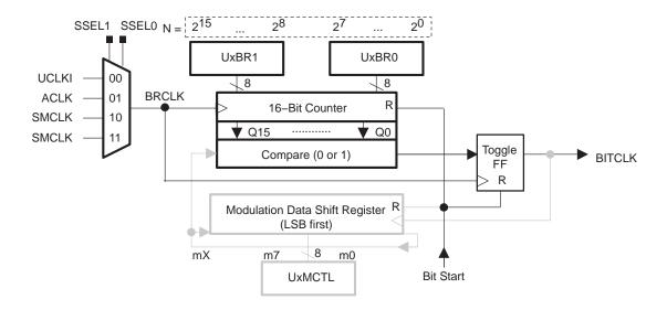
The 16-bit value of UxBR0+UxBR1 is the division factor of the USART clock source, BRCLK. The maximum baud rate that can be generated in master mode is BRCLK/2. The maximum baud rate that can be generated in slave mode is BRCLK. The modulator in the USART baud rate generator is not used for SPI mode and is recommended to be set to 000h. The UCLK frequency is given by:
